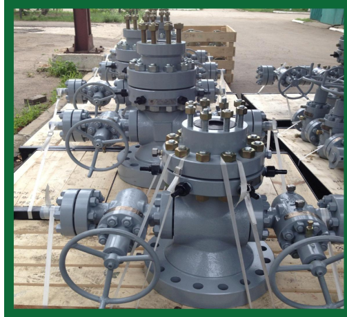
Wellhead & Xmass Tree
